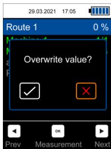
Fig. 36 Overwrite measurement of a measuring spot for current route measurement
